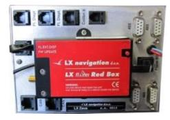
On the rear of the LX Zeus 5.5 and 7.0 there is enough space to install LX Flarm Red Box as an integral part of the system. All connections are plug and play. It is also possible to install any other Flarm compatible devices.
