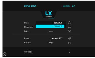
Settings inside Setup menu can always be changed (apart from elevation setting).
