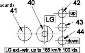
40) Toggle switch for extension and retraction of the electrically operated main landing gear
