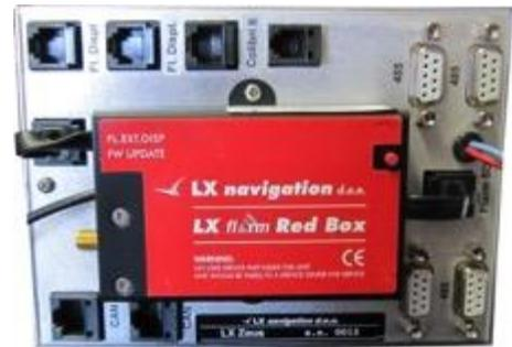
On the rear of the LX Zeus 5.5 and 7.0 there is enough space to install LX Flarm Red Box as an integral part of the system. All connections are plug and play. It is also possible to install any other Flarm compatible devices.
