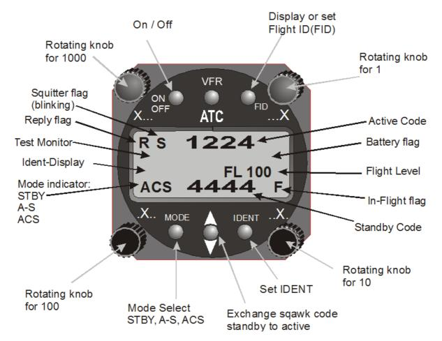
The input elements consist of four rotating knobs and six push buttons.
